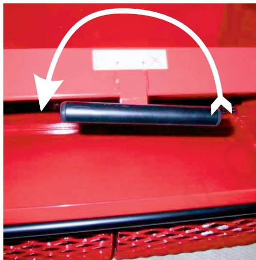
Turn the handle anti-clockwise until the shutter is stopped by the regulating disk. Please note, it is very important that the handle is turned from the closed position anti-clockwise until the shutter is stopped by the regulating disk, if a uniform opening is to be achieved.
